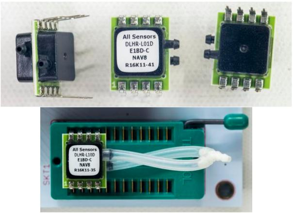
Figure 2. Sensor and connection to Evalboard socket
